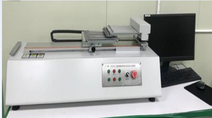
Tabber stringer pull strength testing
