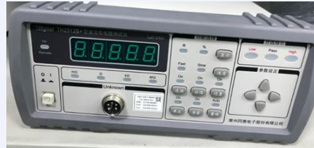
J Box internal resistance loop testing
