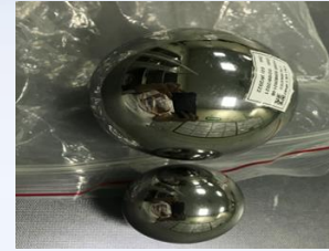
Ball bearing and hammer to test temper glass
